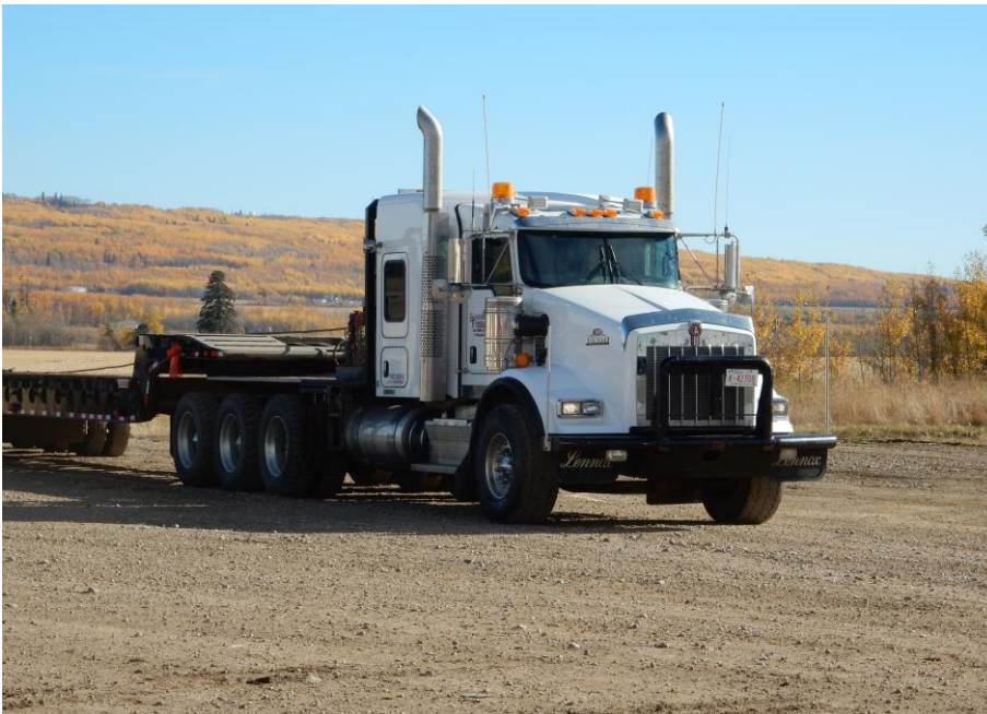
Winch Tractors w/Tri High or Tri Low c/w 50 ton winch
